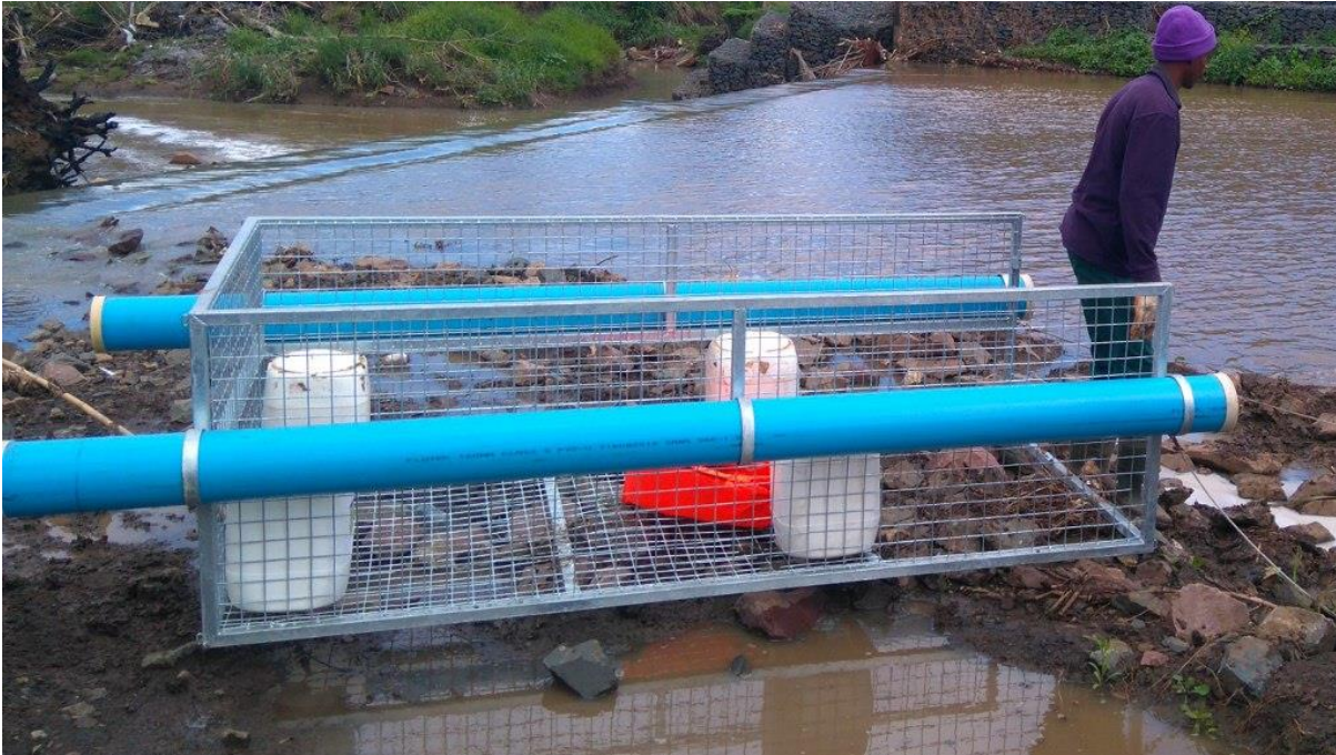
Flotation using both PVC pipes and 20 litre containers.
